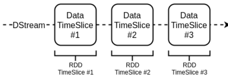
Figure 2.6: DStream representation of multiple RDD
